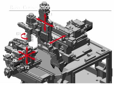
The B-axis machining range for the front spindle has been expanded to 110°. This provides greater flexibility in the machining balance, by reducing the number of tools assigned to back machining for example.
