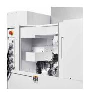
The cutting room door is a flip-up type with a built-in damper, and provides a wide opening for good operating convenience. The larger window also improves visibility when the door is closed.
